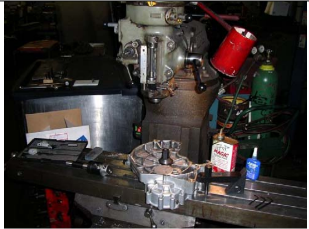
both dowel bores offset and bushed to size
