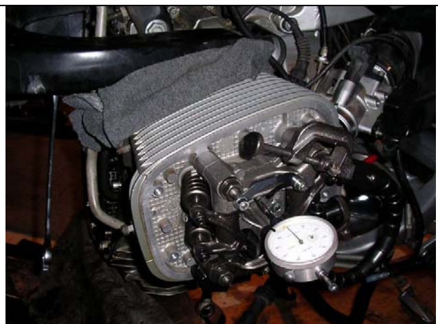
almost done, valve gear installed, and verifying accuracy of TDC mark on flywheel
