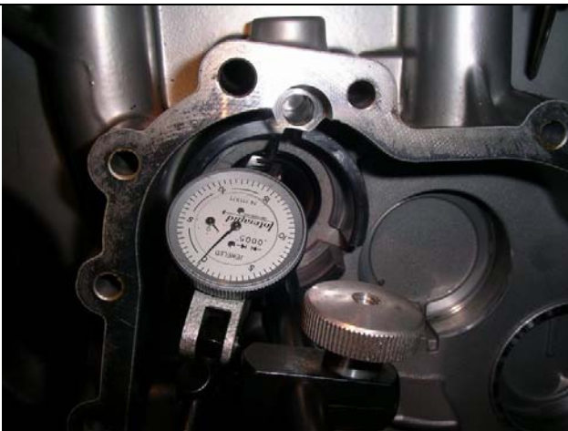
back to zero at 12 o'clock input shaft is 0.0004" to the left of and 0.0003" under the crankshaft
