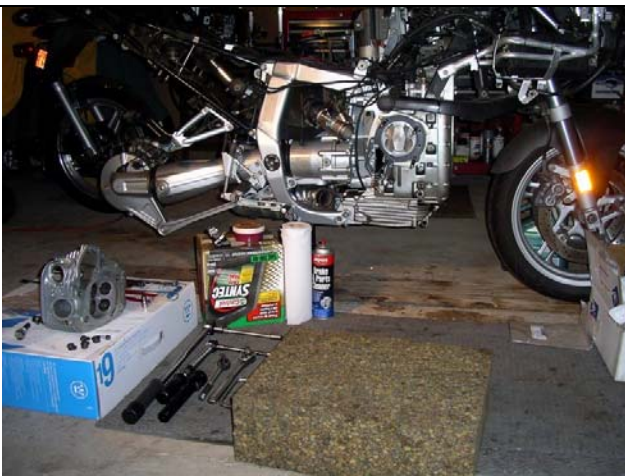
manual says "always install right cylinder first" okay, sure... piston and cylinder installed
