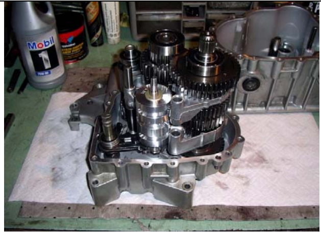
front case took a detour through the oven for a bit so I could slip the bearings into place
