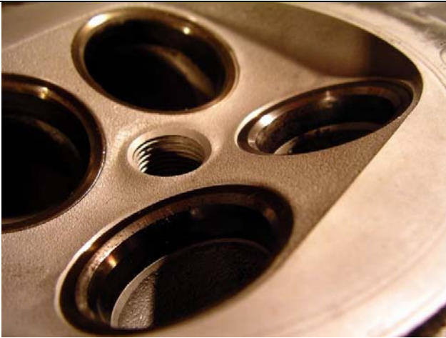
prepping the valve seats
