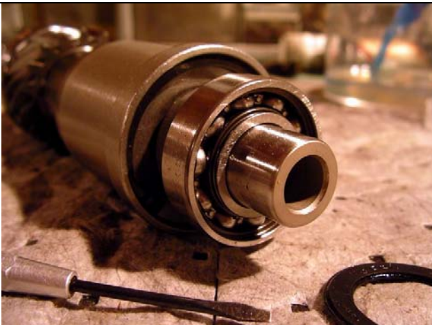
popped the seals off the bearings... not much grease left in there 😬
