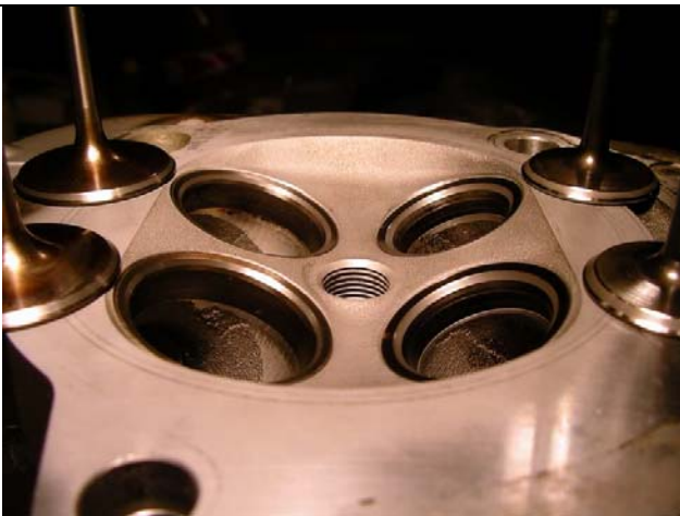
prepping the valve seats
