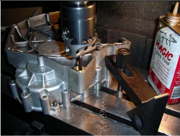
bushing pressed in place, boring inside diameter to 13.52 mm
