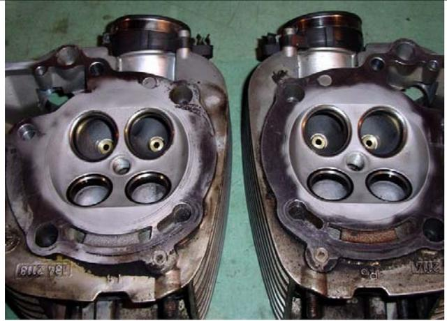
baking soda blasted and washed
