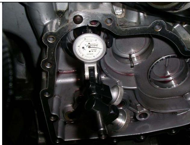
front transmission case installed, test indicator zeroed at 12 o'clock on the input shaft front bearing bore
