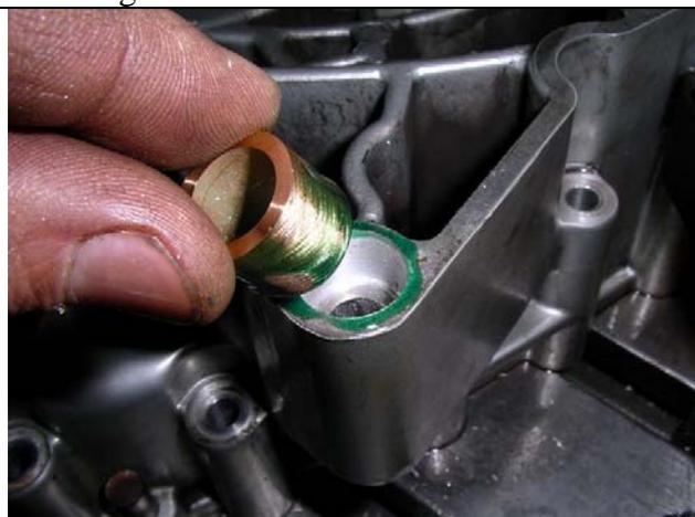
dowel bore in front case bored offset 0.0055" and oversize from 13.52mm to 14.90mm, 15.00mm OD bushing fabbed up, press fit and Loctite 640 to hold it in place
