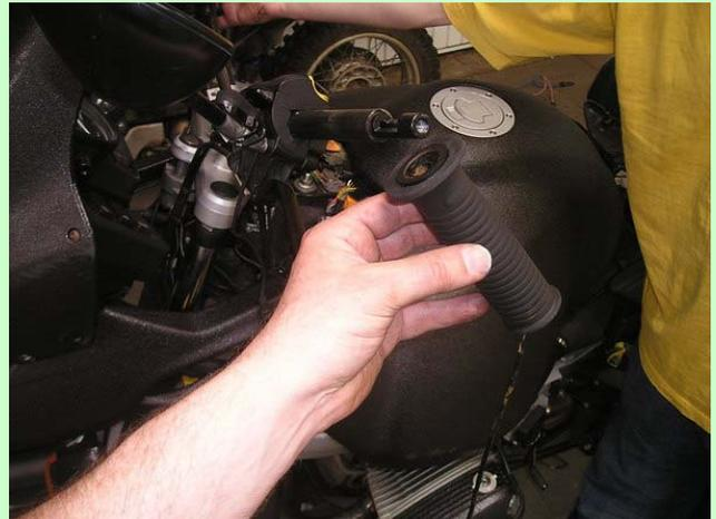
If you replace the steer, you can loosen the grips, unbolt the steer, move it sideways to make some room, slide off the left grip, and then slide off the right grip.
