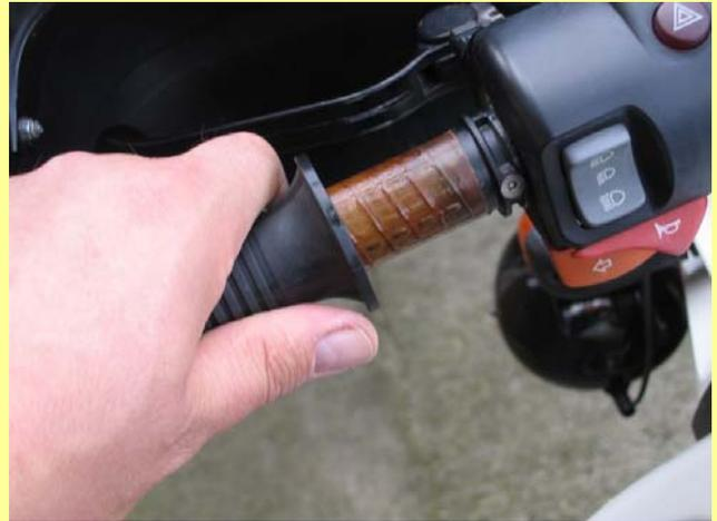
The hairspray went off in about 4 minutes, leaving both grips stuck fast. I did a quick function check, which proved both heated grips were working fine, then replaced the bar end weights and fitted & tightened the countersunk bolts through their washers before declaring the job done.
