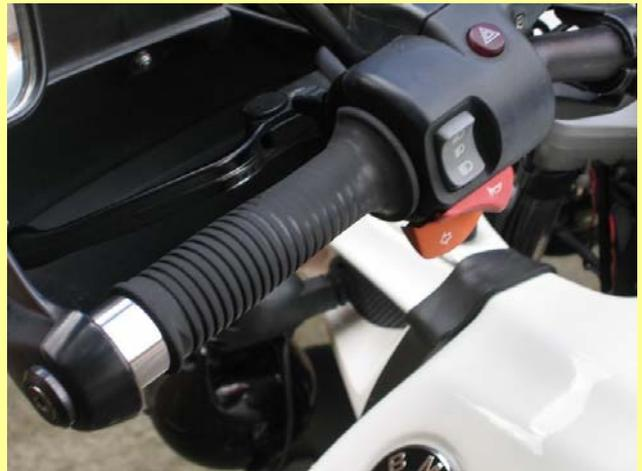
I bought the grips, made by Ariete, from Motorworks, where Kevin told me that, to fit these (pattern) grips, I'd need to buy 2 pairs and use the throttle sized grip on each side, to allow for the extra diameter of the heating element. The two pairs of grips came to a total of just over £20. So, equipped with Allen keys, replacement grips and hair-spray (Tesco's value range - 37p), I set about the task...
