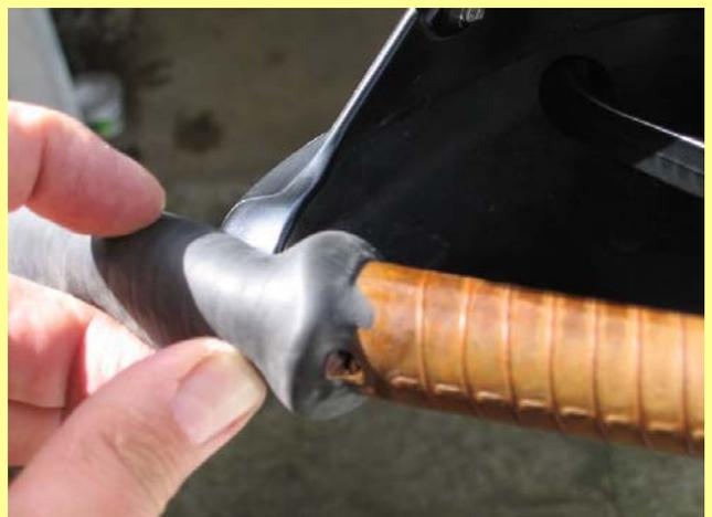
To make life easier I decided to cut most of the rubber off with a craft knife before rolling the remainder back on, in order to try and peel it back from the outboard end.
