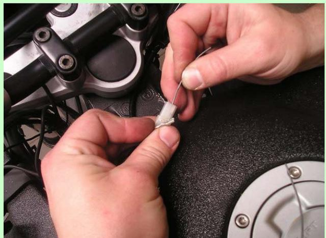
If you take a close look, you can see a sliver of metal angling up from the metal sleeve: that's the tiny hook that you press down to slide the sleeves out of the plastic block. You'll have to push them back up before you push the sleeves back into the plastic block.
