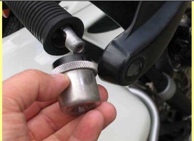
I carefully peeled back the rubber from the switchgear (inboard) end. The grips seem to be glued at both ends, so you have to slowly and carefully let the tension you are putting the rubber under to break the seal of the adhesive.
