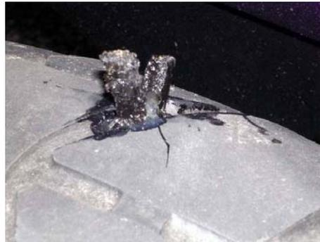
Use a razor blade, or similar tool, to cut the plug level with the tread.
