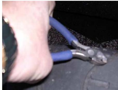
You can see the nail is plenty long enough to go all the way through, and in fact when it was pulled out allowed all the air to leak out quickly. Funny, there was no air leak prior to pulling it out.
