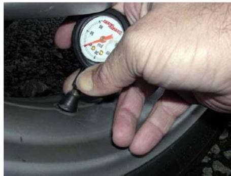
Test the tire for leaks. I used spit, so it looks bubbly, but it isn't, and you can easily see that there are no leaks.
