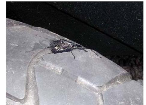
I let the tire sit for 5 minutes with no air in it before I start inflating. This allows the glue to set up some.
