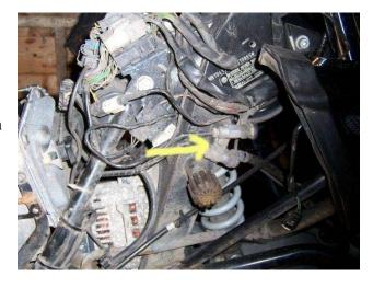
Brake switches were exactly the same shape and size as those that had been removed, so fitting them was a reversal of removing the old ones. The tricky bit was wiring them up.
