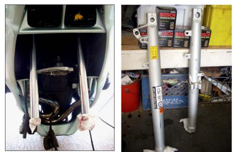
Remove the dust caps by hand , then remove the retainer ring with a small screwdriver. I used an older Craftsman pry bar to remove the seal.
