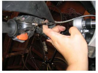
I threaded the new cable alongside the old one, to make sure it followed exactly the same path, to avoid it getting kinked or trapped. I undid both the left and right cables at the throttle bodies.
