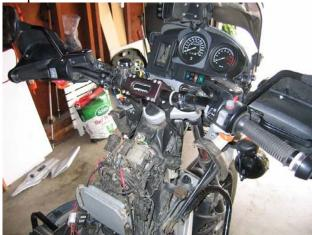
Who have GS may find my bike a little different to yours. I don't have ABS, so there's a big gap ahead of the battery, where the ABS pump would live; I have an alarm and a Techlusion 259, as well as various other electrical bits fitted.
