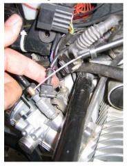
Undo the 10mm locknut, unscrew the adjuster and, after feeding the cable through the gap in the plate, disconnect the spring clip on the inner side of the throttle body to release the cable. You have to do this by feel, but you'll get the idea when you try it.
